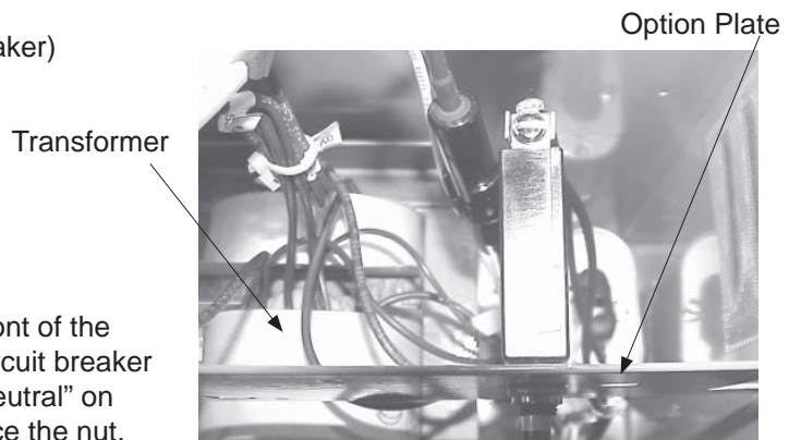
Fig. 2-11, Input Circuit Breaker Installed in Option Plate
