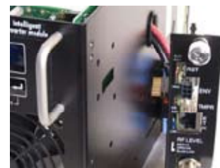
Mounting transponder to the XM2 Inverter Module
