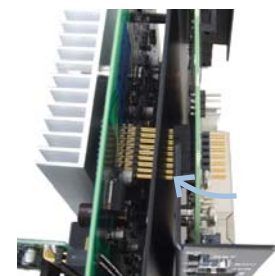
Fig. 6, Connecting the DPM to the Inverter Module
