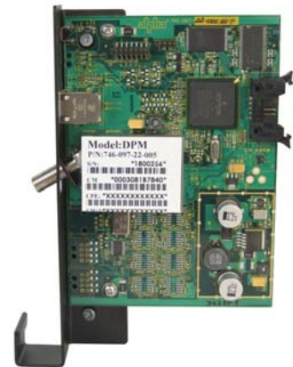
Fig. 3, Captive Screw /MAC Address Label location
