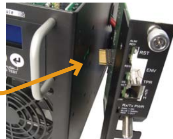
Fig. 8, Connecting the Communications Module to the Inverter Module
