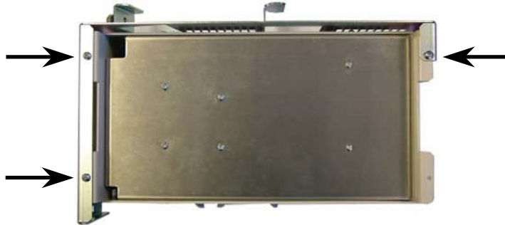
Figure 16–Location of FMPS mounting bracket screws
