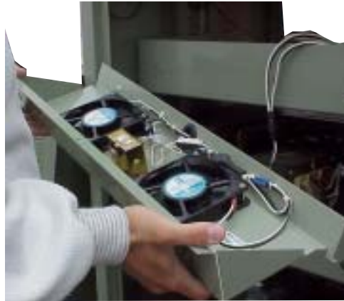
Figure 4-14; Cooling Fan Panel
