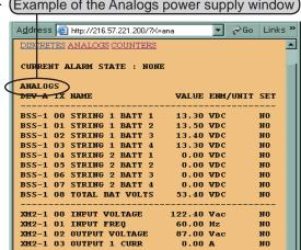
**Method Two:** To check connectivity and verify power supply data, the XP-DSM can be accessed with SNMP. Check data within the psIdent MIB branch of the SCTE-HMS Tree by performing anzzz SNMP MIB walk to the SCTE-HMS-MIB branch 1.3.6.1.4.1.5591.1. Verify that power supply data measurements are present.
