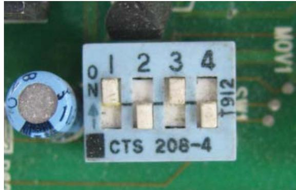
Fig. 2-2, A2304 Dip Switch Configuration
