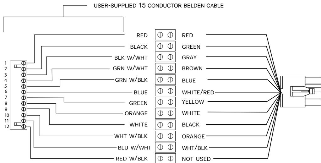
Fig. 4-4, Standard Transponder-to-ACM interconnect cable, **remote** applications
