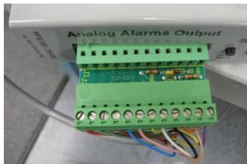
Fig. 4-2, Alarm Filter Board
