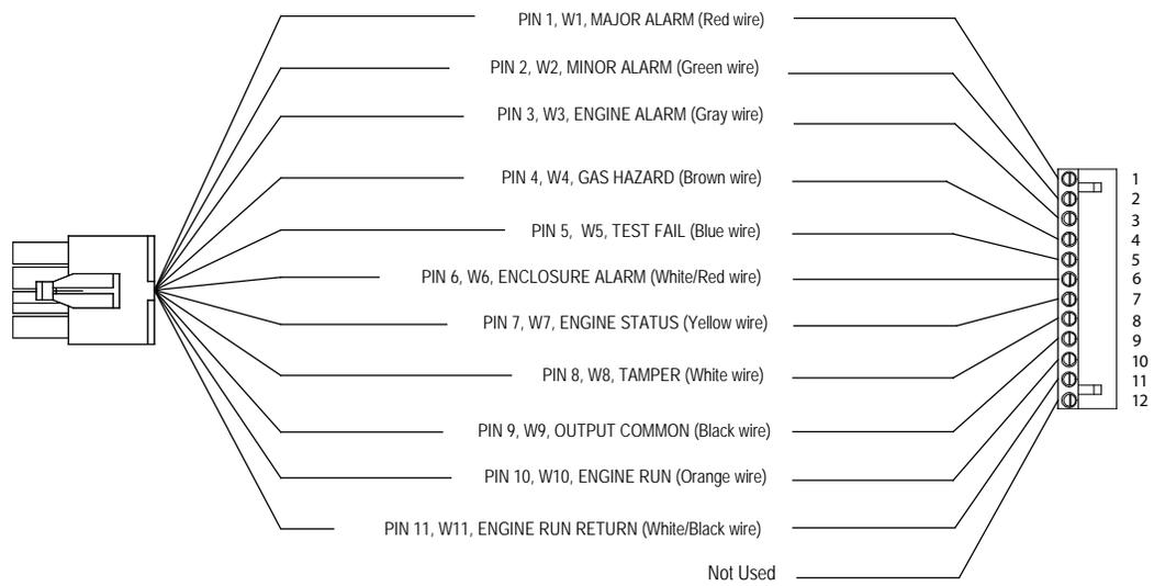
Fig. 4-3, Standard Transponder-to-ACM interconnect cable, **collocated** applications
