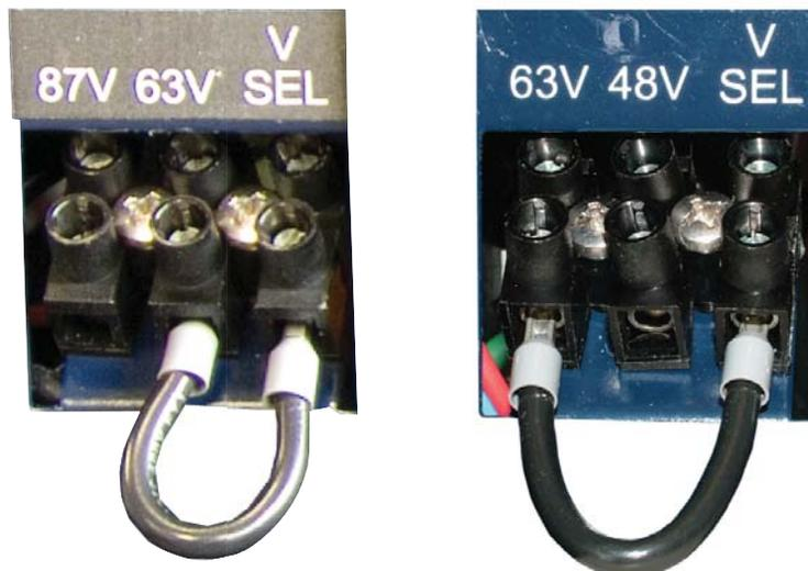
Fig. 4-2, Transformer Output Tap Connectors
