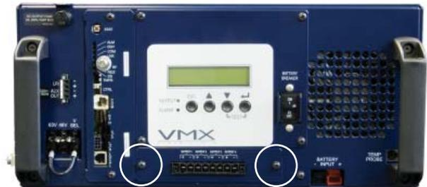
2. Pull the connector plate clear of the chassis and disconnect the five wires.
