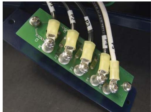
3. Connect the wires to their appropriate terminals on the coax cable connector. The neutral wire mounts below the board.
