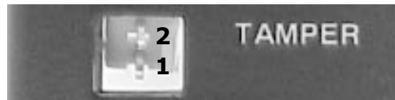
Figure 1-11; Tamper Switch Pin Arrangement
