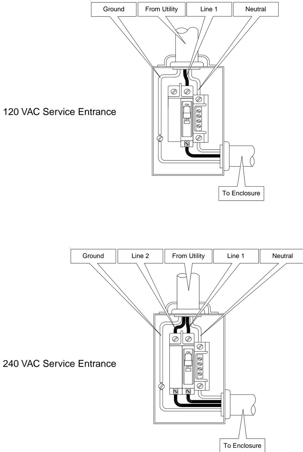
Figure 2-3 Typical Service Entrance Wiring
