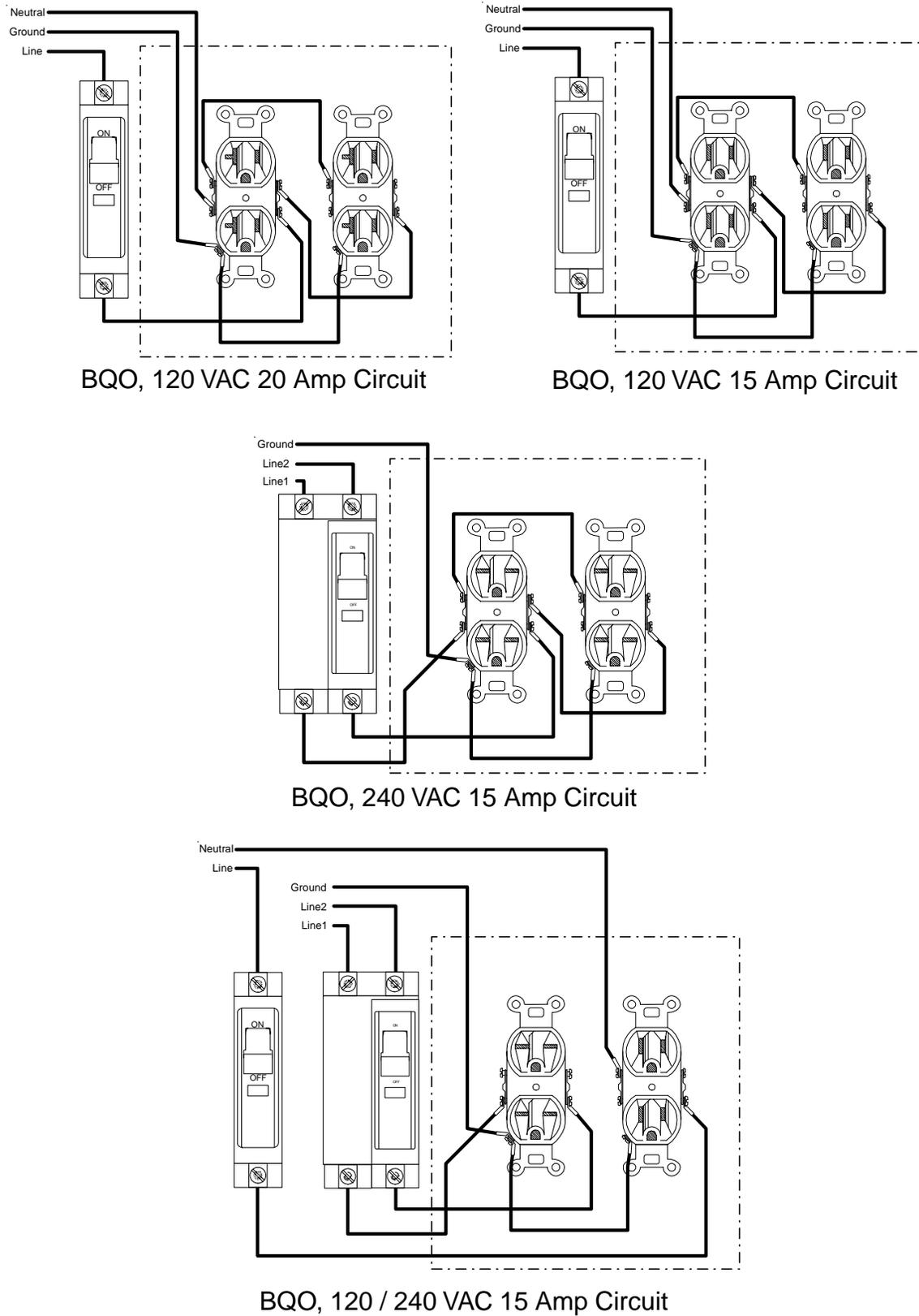
Figure 2-4 Breaker-Quad-Option Wiring
