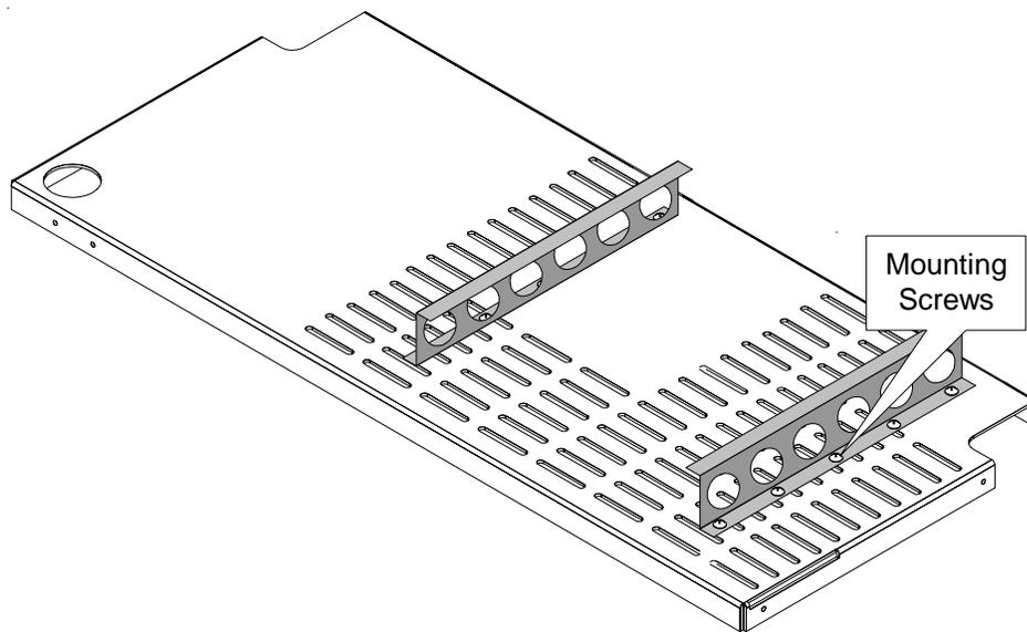
2. Place the power supply on the top tray, ensure that the feet are OUTSIDE the rails and the power supply rests level.
