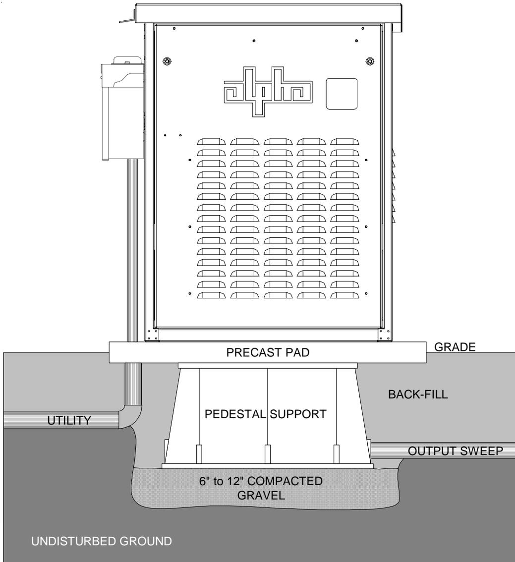
Fig. 1-3 Enclosure installed on a model PS2 support
