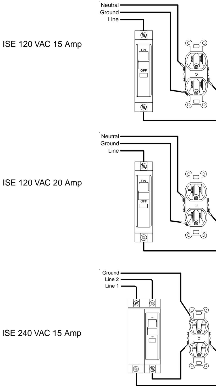
Figure 2-2 Typical ISE Receptacle Wiring
