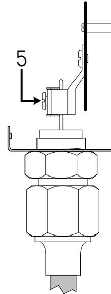
4. Insert the Coaxial Termination into the Output Port on the bottom of the SPI.
