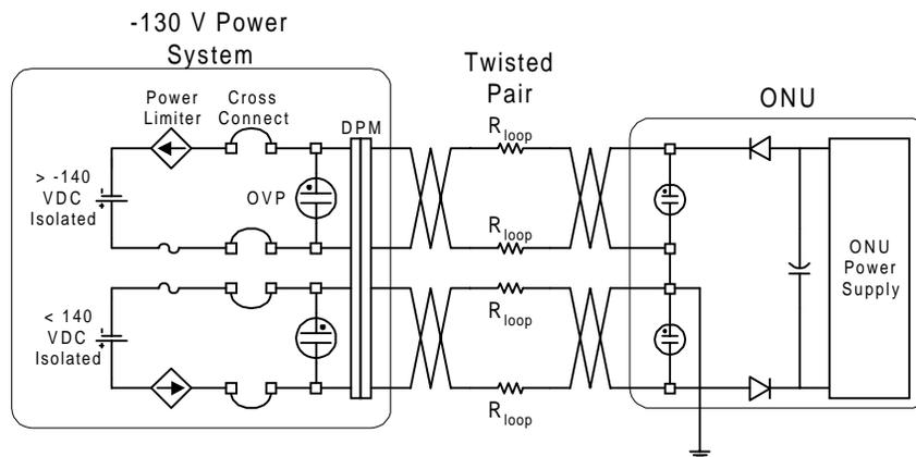
Figure 6.  $\pm 130\text{V}$  Twisted Pair Powering Loop
